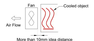
Keep some distance, between the object to be cooled and the inlet of the fan
